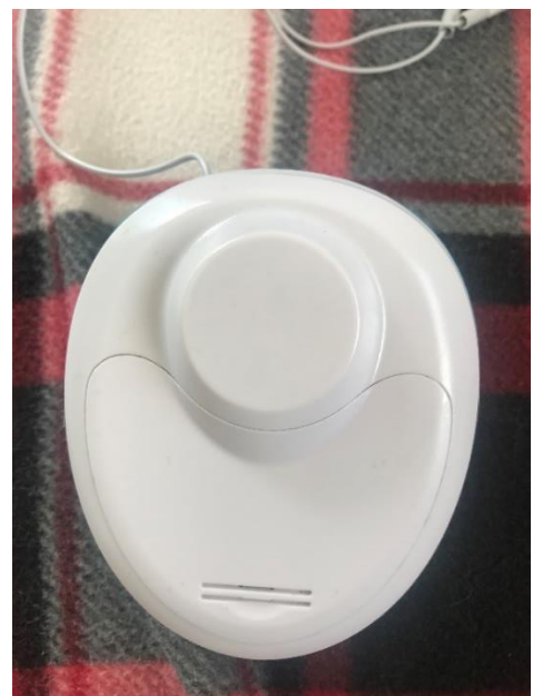
Figure 3: Another type of handheld fetal Doppler marketed to women. This type does not have a built-in display or speaker, and requires the user to attach headphones to hear sound. Audio can be recorded by this device and can be uploaded to the user’s computer via a USB cable.
