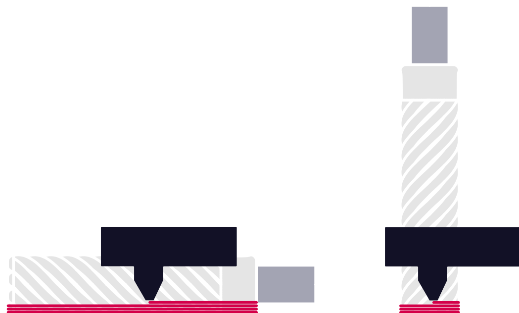
Figure 76. Horizontal and vertical print orientations.
