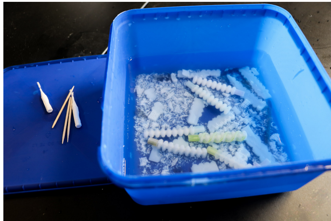
Figure 22. Support material cleaning setup.
