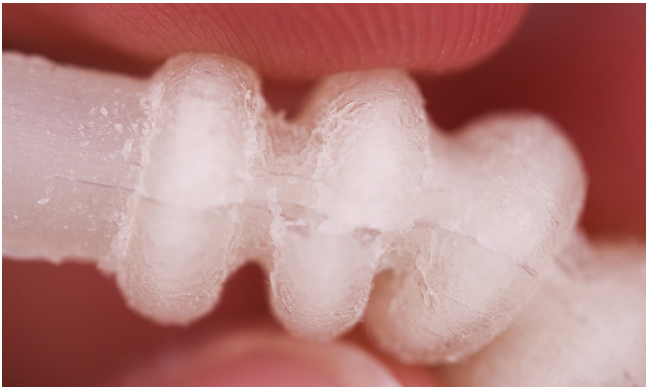
Figure 96. Print set 1 material tear.
