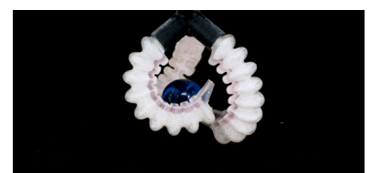
Figure 90a - 90g. Gripper print geometry and demonstration gripping various objects.
