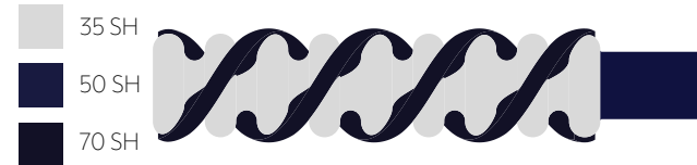
Figure 27a - 27g. Actuator 3.02 geometry and inflation sequence.
