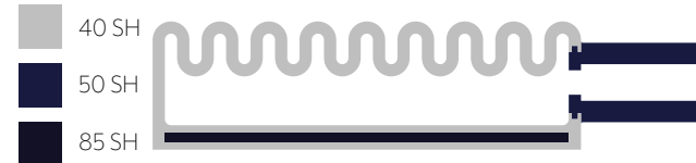
Figure 35a - 35g. Actuator 2.04 geometry and inflation sequence.
