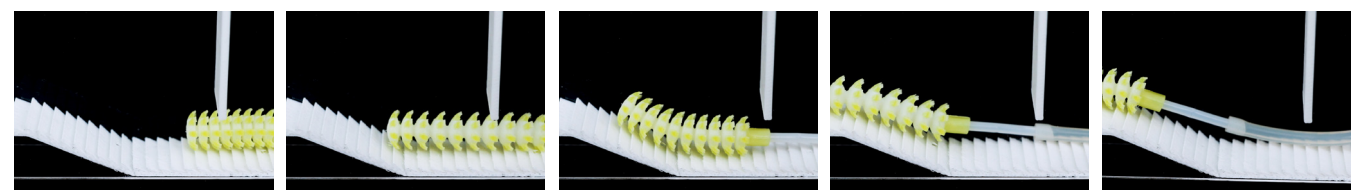
Figure 91a - 91i. Extension/adhesion print geometry and locomotion along a course.
