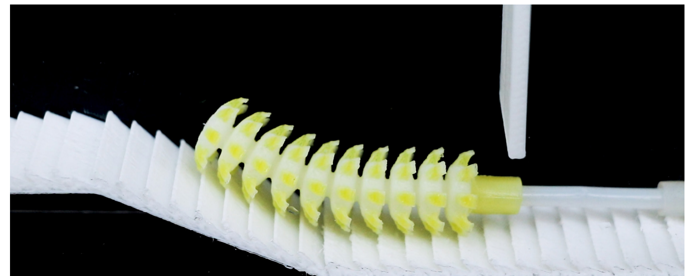
Figure 98. Locomotive extender traversing an obstacle course.
