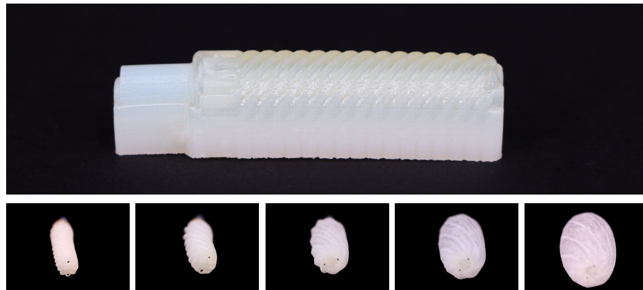
Figure 71a - 71g. Actuator 3.12 geometry and inflation sequence.
