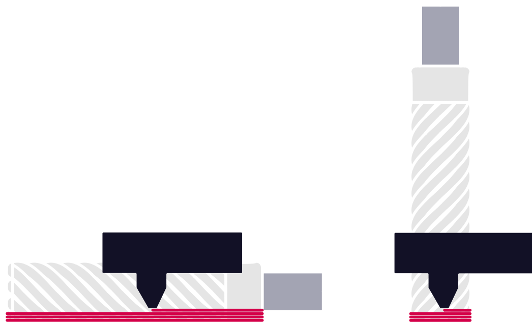
Figure 70. Horizontal and vertical print orientations.
