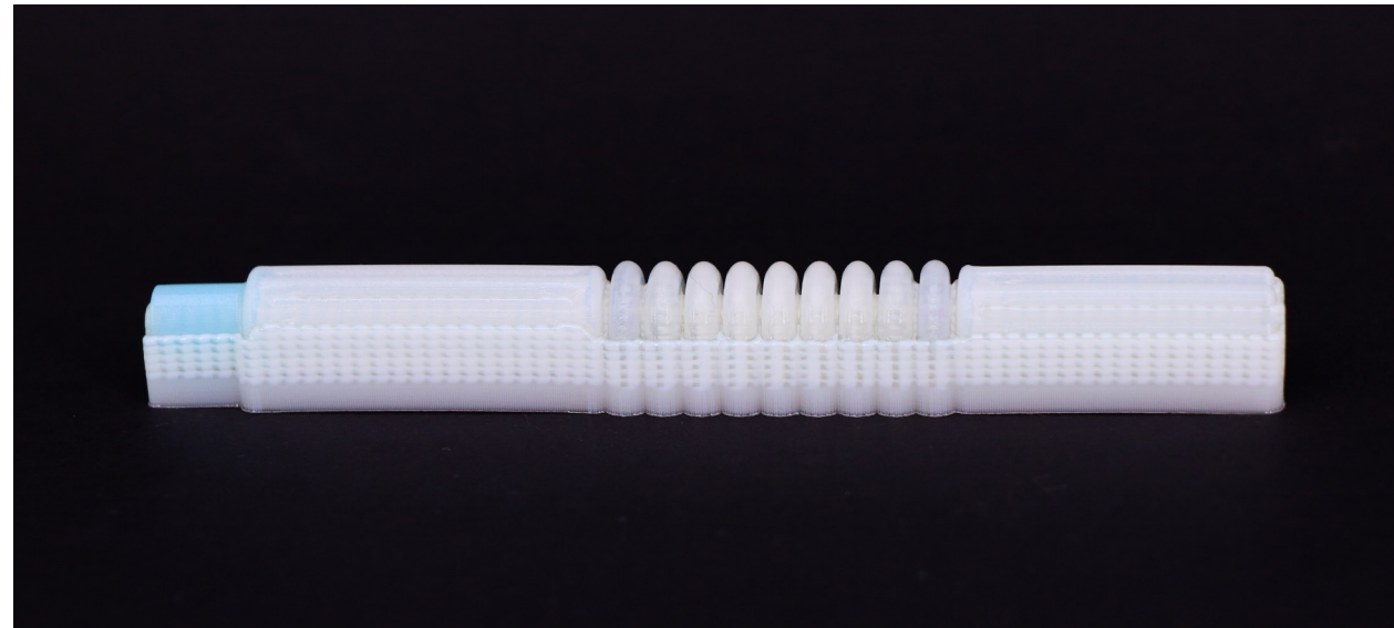
Figure 53a - 53b. Actuator 5.02 geometry.
