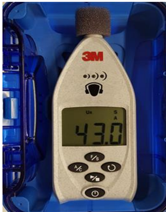
Figure 92: Image of the 3M Sound Detector SD-200 Sound Level Meter
