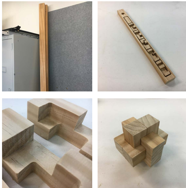
Figure 22. The digital fabrication process of a six-piece Burr puzzle using a CNC machine.
