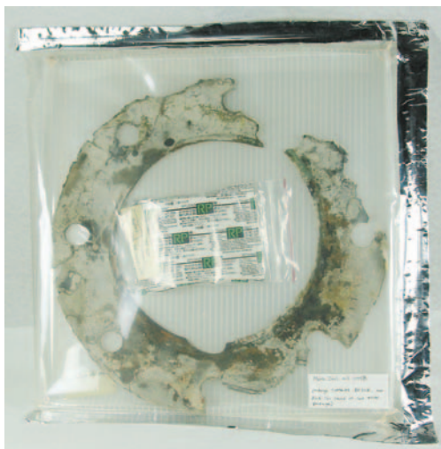
Fig. 11. The RP-K 20 system in use on a rubber gasket. The gasket is enclosed in an Escal bag and heat sealed. Aluminum type is then placed around the seal. The RP is in the center in a polyethylene bag. A coroplast board is placed under the gasket for support.
