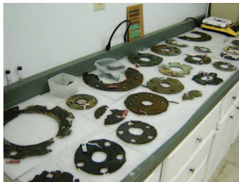
Fig. 7. Part of the collection of rubber gaskets from the Monitor steam engine. Notice the variety in size and condition.
