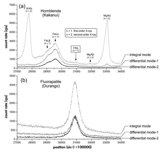
**Figure A2. 1.** Spectral scans for two EPMA standards with varying pulse height analysis (PHA) settings. a) Hornblende Kakanui standard (USNM 143965). b) Fluorapatite Durango (USNM 104021). Changing the PHA conditions removes the interference on  $FK\alpha$  from the MgK $\beta$  line, and lessens the interference from the FeL $\alpha$  line (a), without depressing FK $\alpha$  (b). Sourced from Zhang et al. (2016).
