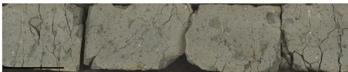
Fig. 4.11: Facies 6 – weakly to well-stratified diamictite. Here weak stratification is indicated by occasional alignment of clasts (core 27, section 3). Stratigraphic top is to the left, and the scale bar is 5 cm long.
