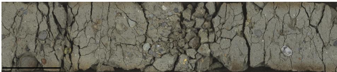
Fig. 4.10: Facies 5 – massive diamictite (core 27, section 3). Stratigraphic top is to the left and the scale bar is 5 cm long.
