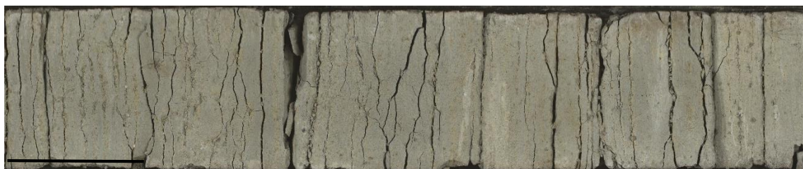
Fig. 4.9: Rhythmically interlaminated mudstones with silt-/sandstones. Brown coloured beds are the fine sandstones, and grey beds are the mudstones (core 24, section 2). Stratigraphic top is to the left, and the scale bar is 5 cm long.
