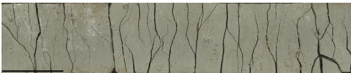
Fig. 4.6: Facies 1 – mudstone (core 17, section 3). Note the lack of clasts. Stratigraphic top is to the left, and the scale bar is 5 cm long.
