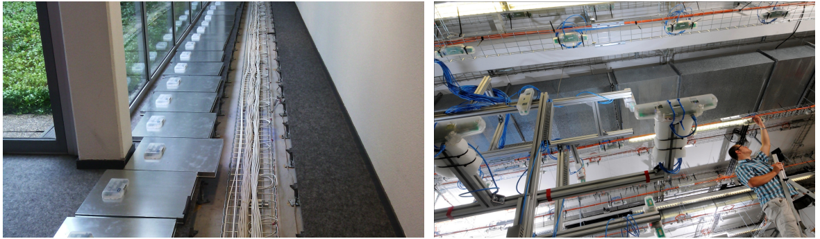
(a) Deployment of nodes in the IoT-LAB Grenoble site (b) IoT-LAB nodes in the Grenoble Senslab space
